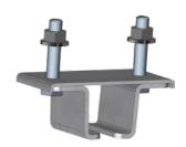
This bracket mounts to a customer-supplied angle iron at two points to hang the C-Track. The separate "Z" clamps allow mounting of the C-Track Channel without needing to feed it through the hangers from the end. The clamping action of the support bracket eliminates the need for a separate anchor.
