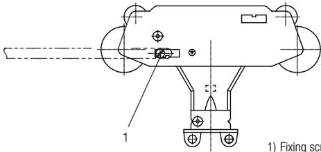
1) Fixing screw for current strip (do not pull tight)
