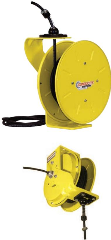
This reel can be used to power moving machinery or used by hand use a customer-installed cable-end accessory. If the accessory weighs over two pounds (0.9 kg), please contact the factory. Reels come with ball stop and various cable types; see Table A on page 9. Three-conductor 110 volt reels come with six foot feeder cord and NEMA 2 molded plug. Four conductor reels are rated NEMA 4 (IP56) for indoor or outdoor use.
