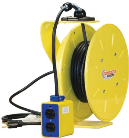
This version of the 1200 Series PowerReel comes with a factory installed receptacle box as noted below. Boxes are yellow, heavy-duty molded TPE (thermoplastic elastomer) - oil resistant and impervious to most chemicals. Includes internal cord grip. Reels include six-foot feeder cable with molded plug - rated NEMA 2 for indoor use. GFCI (Ground Fault Circuit Interrupter) models include the GFCI as part of the plug on the feeder cord.
