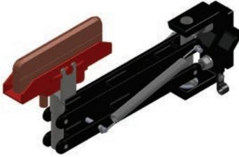
21” long pigtails, 4 AWG, are supplied on the collector. Customer supplied wiring connects to the collector pigtail with in-line connectors. **Used on 500A conductor bar only.**
