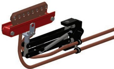
42” long pigtails, 2 AWG, are supplied on the collector. Customer supplied wiring connects to the collector pigtail with in-line connectors. **Used on 700A - 1500A conductor bar only.** Note that the 300A version is the same as the 200A, except with an extra tension spring on the arm.
