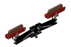
42" long pigtails, 2 AWG, are supplied on the collector. Customer supplied wiring connects to the collector pigtail with in-line connectors. **Used on 700A - 1500A conductor bar only.** Note that the 600A version is the same as the 400A, except with one extra tension spring on each arm.
