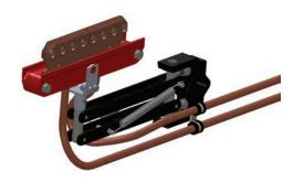
42" long pigtails, 2 AWG, are supplied on the collector. Customer supplied wiring connects to the collector pigtail with in-line connectors. **Used on 700A - 1500A conductor bar only.** Note that the 300A version is the same as the 200A, except with an extra tension spring on the arm.
