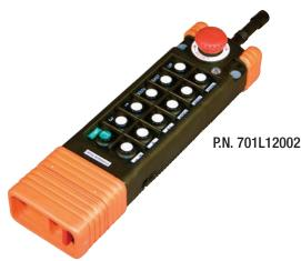
The L12 Series is a 2-speed transmitter with twelve buttons for control of up to 5 motions. FCC 310-320 Mhz AC models only. Each kit includes receiver, one or two transmitters, four batteries, strap, legend sheet for each transmitter, spare key, spare fuse kit, and instruction manual. This radio has programmable operation; contact Conductix-Wampfler to discuss your application needs.
