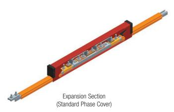
Expansion Sections are used at all structural expansion joints and for systems longer than 492 ft. (150m) to allow for thermal expansion / contraction of the bar. The maximum gap of the Expansion Section is 2.0" (50 mm). The Expansion Section is 14' 9" (4.5 m) long and is installed in place of one length of conductor bar.
