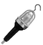
Ideal when a hand lamp needs to be used in a hazardous location. Light-weight construction. Features non-sparking aluminum guard with full swivel hook and high impact glass reinforced phenolic handle. Resists heat up to 300° F. Accepts up to 14/3 SOOW-A cable. 100 Watt, 120 Volt.
