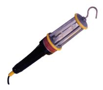
Ideal when a hand lamp needs to be used in a hazardous location. Light-weight construction. Features non-sparking plastic guard with full swivel hook and high impact glass reinforced phenolic handle. Resists heat up to 300 degrees F. Accepts 16/3 SOOW-A cable. 13 Watt, 120 Volt
