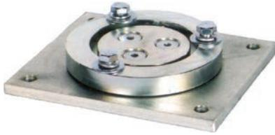
The Pivot Base allows reels to rotate up to 345 degrees left-to-right. The unit bolts to the base of the reel in the field (see page 24 for more details). Also fits 1200 Series reels.
