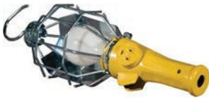
The HSR has a high impact yellow handle with recessed on/off switch and 15 amp, 125 volt outlet on the side. Features a grounded steel reflector cage with swivel hanger. Accepts up to 14/3 SJ00W-A cable. 100-watt rough service bulb not included.
