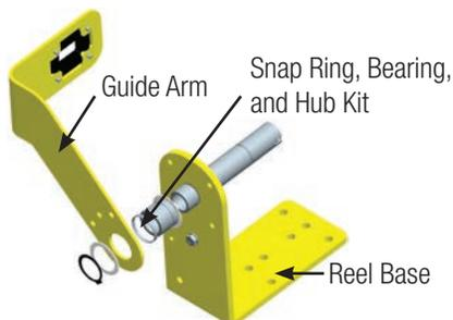
The Flop-Over Guide Kit consisting of special hub, snap ring, and bearings. The kit modifies the standard stationary guide arm to let it freely pivot around the shaft hub. Ideal for overhead reels that require a back and forth payout. Only for 1400 Series.
