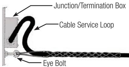
Cable Grips (or Kellems Grips) relieve the concentrated strain at the cable termination point, thereby increasing cable life. Grips are recommended for all applications. In most installations, the eye of the cable grip is connected to an eye bolt or U-bolt. Allow for a cable service loop to minimize the strain on the cable.
