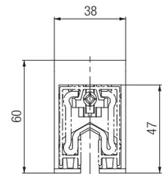
End Caps are used as a rail terminator and contact protection and are fastened to the rails using clamping screws.
