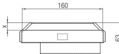
The copper graphite shoe is protected by a plastic insulator, so that accidental contact with live parts of the engaged Current Collector is not possible.
