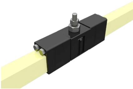
The rails are fixed in one place with Anchor Clamps and can expand freely from that point out. The fixed point is mainly for single feed applications attached close to the power feed or in the center of the conductor rail system. If multiple fixed points are planned, for example at intersections or curves (natural fixed point), the segment between the fixed points must be decoupled using Expansion Units. Clamps are fastened with a clamping cone on the rail insulator.
