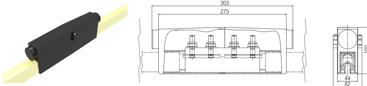
Rails are connected using compact screw connections. The rail connections must have exposed metal on all contact surfaces and be coated with a thin layer of contact grease (Part no. 080021) to protect against corrosion. When mounting clamping screws, use a torque wrench to achieve correct tightening torques.
