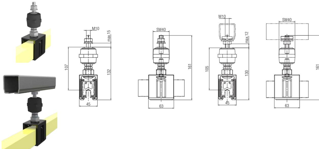
Suspension is carried out using freely swivelling clip-on Hanger Clamps that are self-aligning and permit low-friction slipping in case of thermal expansion. Hanger Clamps are available with hex nuts or square nuts for the mounting of Support Arms / C-rail (see installation accessories).
