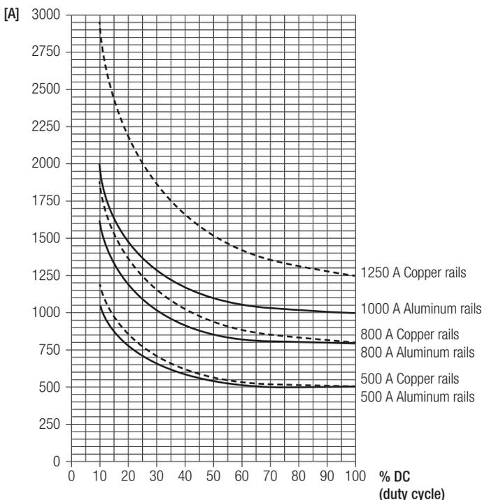
The load current of the conductor rail can be increased for shorter duty cycles.
