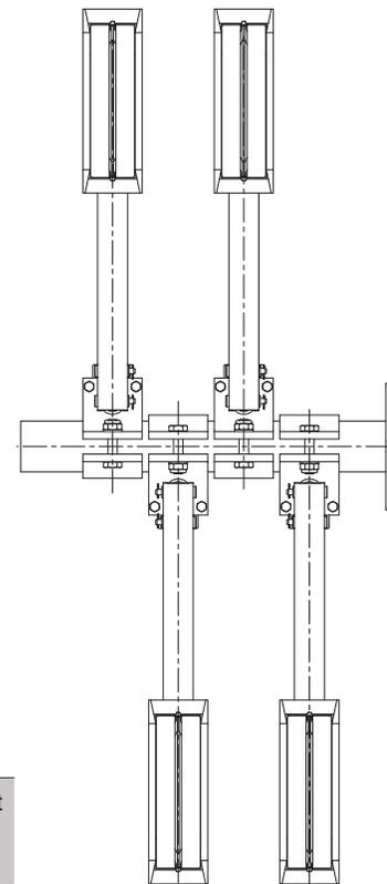
For installations without transfer points the current collectors for vertical and horizontal operation can be staggered. This way the center distance between two conductor rails is reduced by 10 mm.
