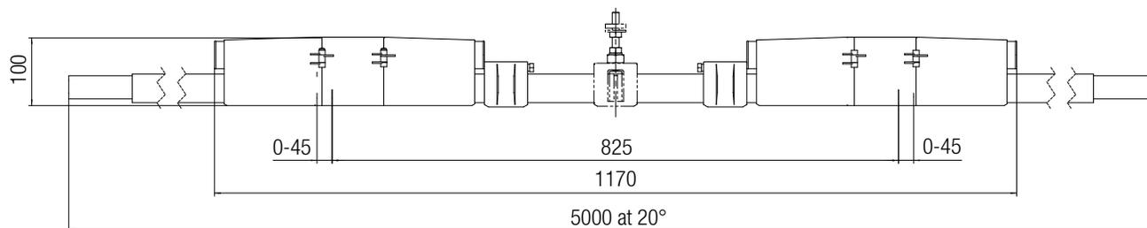
To compensate for changes in length due to temperature for systems > 200 m or segments connected between two fixed points such as Pickup Guides on both ends of the segment, or in curves (natural fixed points), expansion elements are needed to absorb the change in length. The expansion element has two expansion points, each of which can absorb 25 mm of expansion. The expansion elements / expansion unit parts are, like the rails, designed as 5 m standard components.
