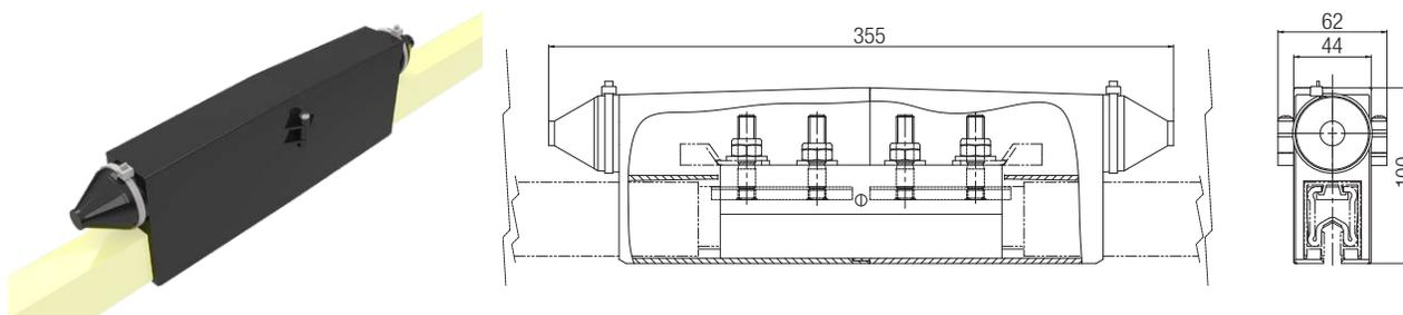
The power feed uses a power connector; these replace the normal rail connectors. Electrical connection is provided using projecting bolts and tubular cable Lugs (cable and cable lugs not included; please order separately).
